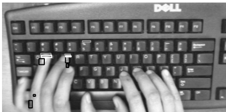
(a) Hand tracking analysis. Rectangles identify regions in movement. Black rectangles are used for movements in the hands regions, grey rectangles for keys, white rectangles for regions where both hand and key movement happens. These rectangles identify likely key presses.
